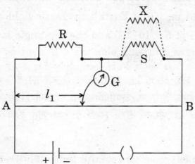
When an unknown resistance X is connected in parallel with the resistance S, the balance point shifts to a distance  $l_2$ . Find the expression for X in terms of  $l_1$ ,  $l_2$  and S.
